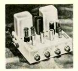
impedance of conventional output circuits. Damping factor control permits perfect match of amplifier output im-pedance to loudspeaker's critical damping resistance. Output 20 watts rated, 40 watts on peaks. Frequency response  $\pm$  0.1 db, 20-20,000 cycles at 20 watts.
