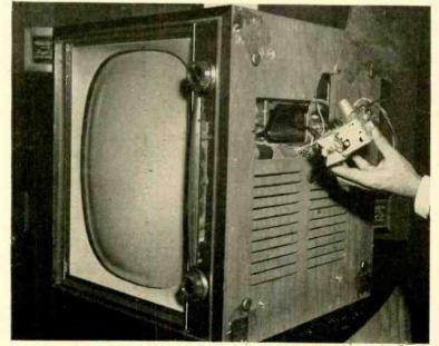
U.h.f. Tuner-Adapter has been announced by Philco (see photo). The unit consists of a u.h.f. tuner, adapter cables and plugs, a planetary tuner driving assembly and mounting hardware. A feature of the adapter is that it can be installed without removing the chassis or cabinet back.
