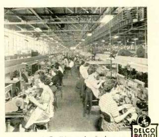
Each RF and IF coil is wound under the supervision of a skilled operator, and each is tested at several points along the production line. This painstaking cure is what gives a high IQ to Delco Radio Coilz.
